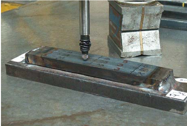
Fig. 3 Measurement of deflections on triplet of specimens welded to supporting plate
