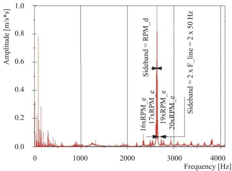
Fig. 3 The acceleration spectrum of motor B, at 146 Hz
