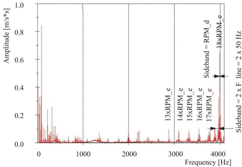
Fig. 4 The acceleration spectrum of motor B, at 221 Hz
