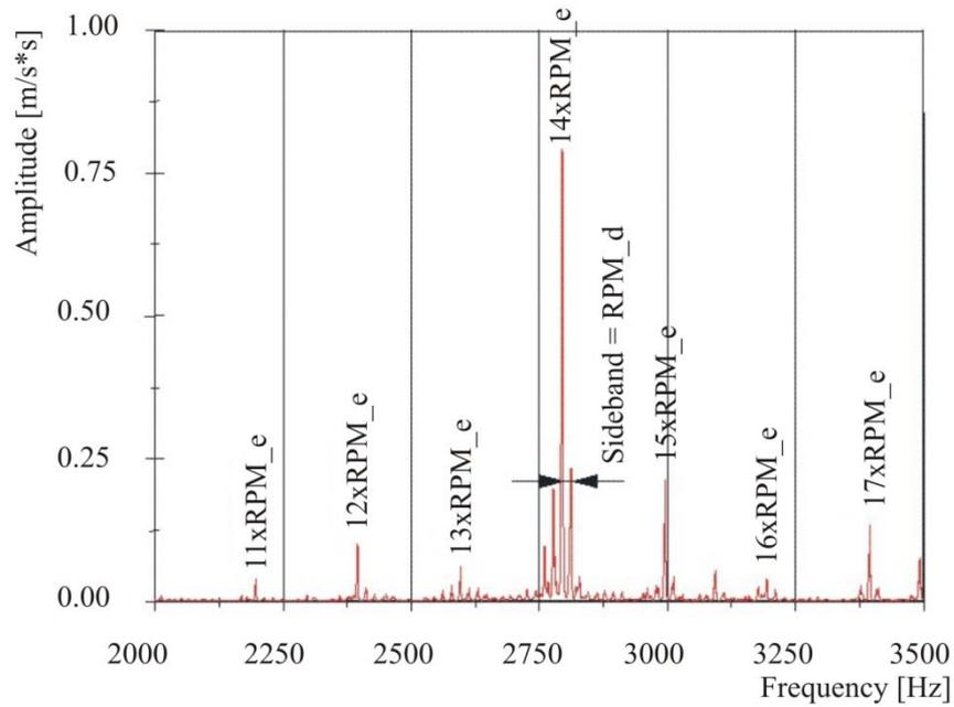
Fig. 2 The acceleration spectrum of motor A, at 199 Hz
