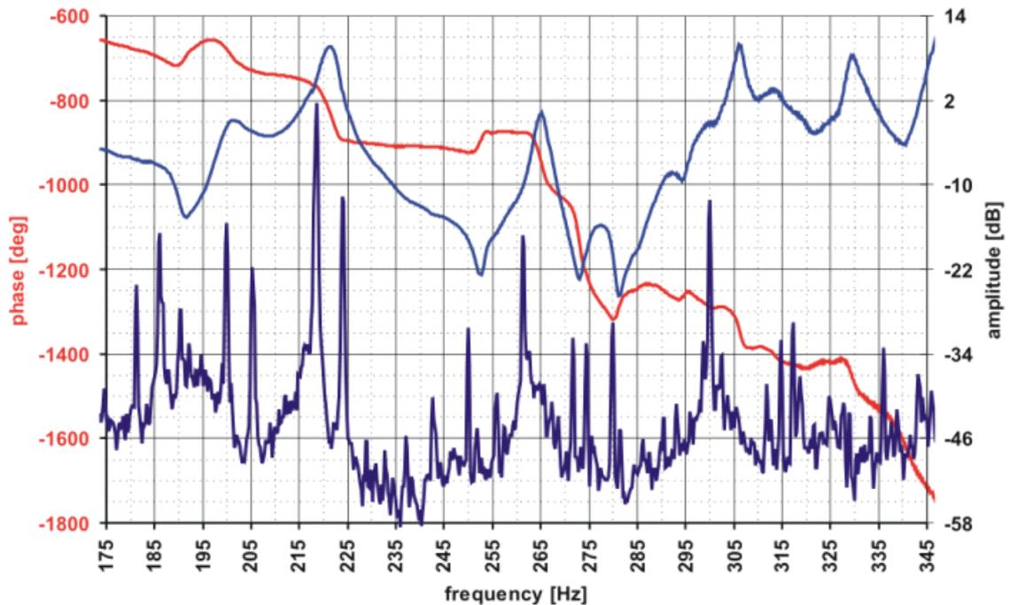
Fig. 8 The comparison of acceleration spectrum and amplitude FRF on the sheet of cabinet
