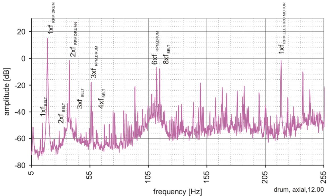
Fig. 5 The frequency spectrum of acceleration on the drum in axial direction
