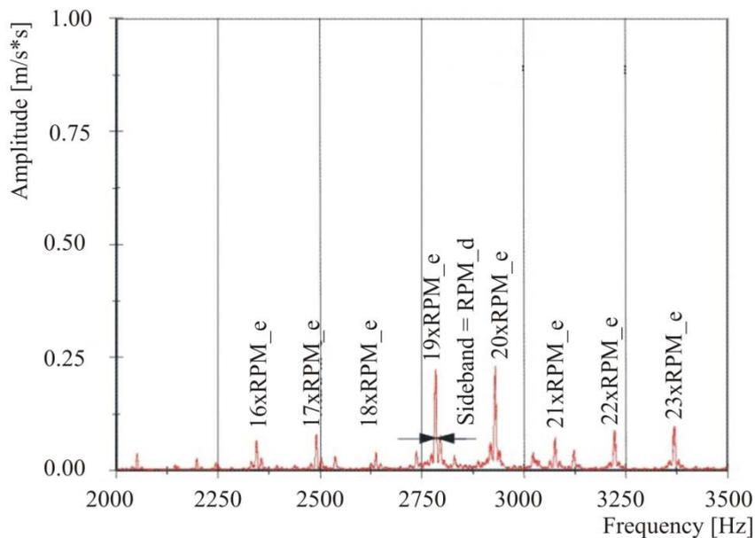
Fig. 1 The acceleration spectrum of motor A, at 149Hz
