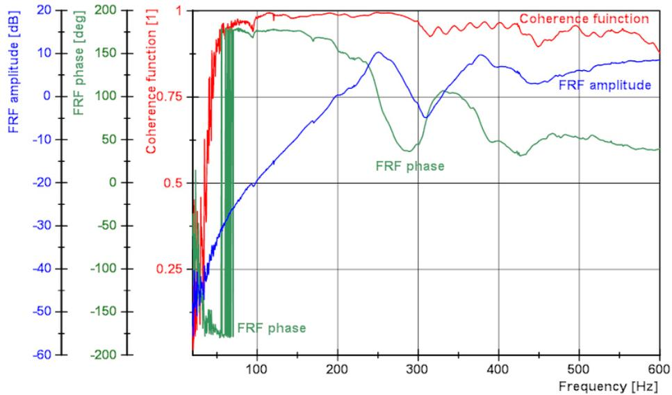
Fig. 7 The FRF of shock absorber, natural frequency at around 250Hz
