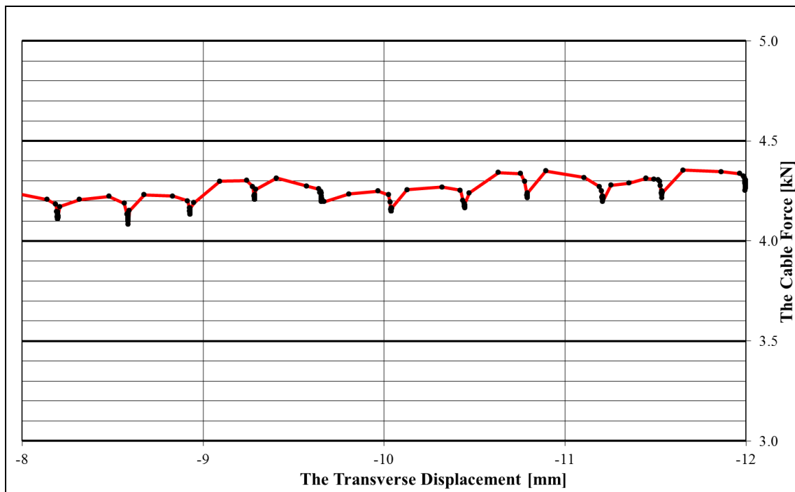
Fig. 4 The edge cable placed in a fabric pocket (the point No. 1) – the dependence of the evaluated cable force on the transverse displacement.
