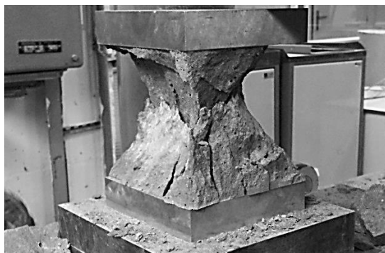
Figure 4 Typical shape of specimen after testing
