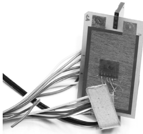
Figure 3. Piezoelectric patch with applied strain gauge rosette.
