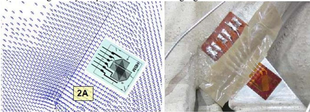
Fig. 3: Analysis of strain directions and installation of strain-gauge rosette at the point 2A
