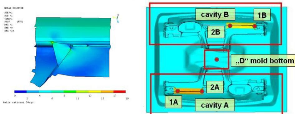
Fig. 2: Example of results of FE analysis and distribution of points of maximal stress
