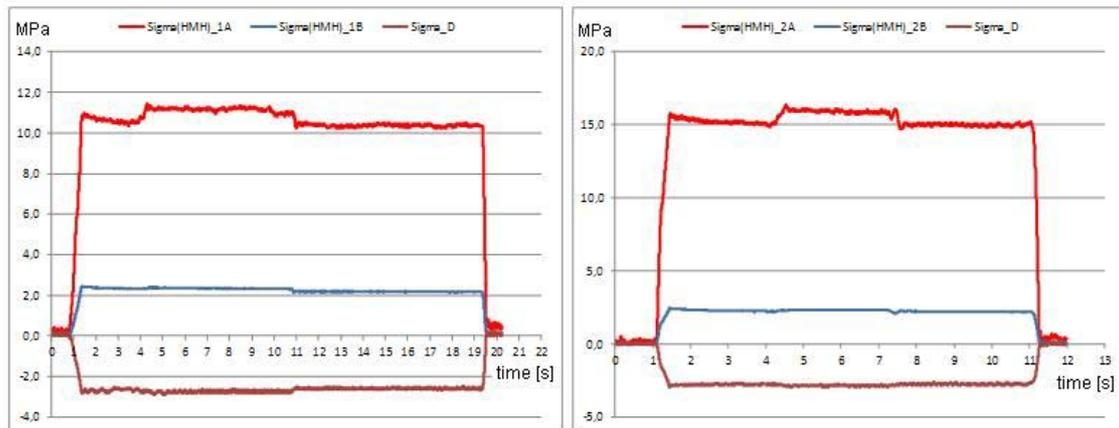
Fig. 4: Time behaviour of  $\sigma_{\text{HMH}}$  at measured points when fixing the inner bucket
