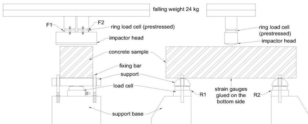
Figure 2: Sample position and instrumentation of the supports and impactor.
