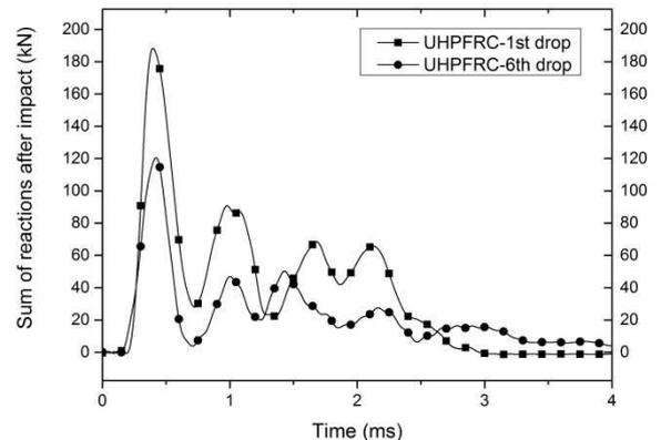
Figure 5. Reaction response of UHPFRC specimen, comparison between 1<sup>st</sup> and 6<sup>th</sup> hit.
