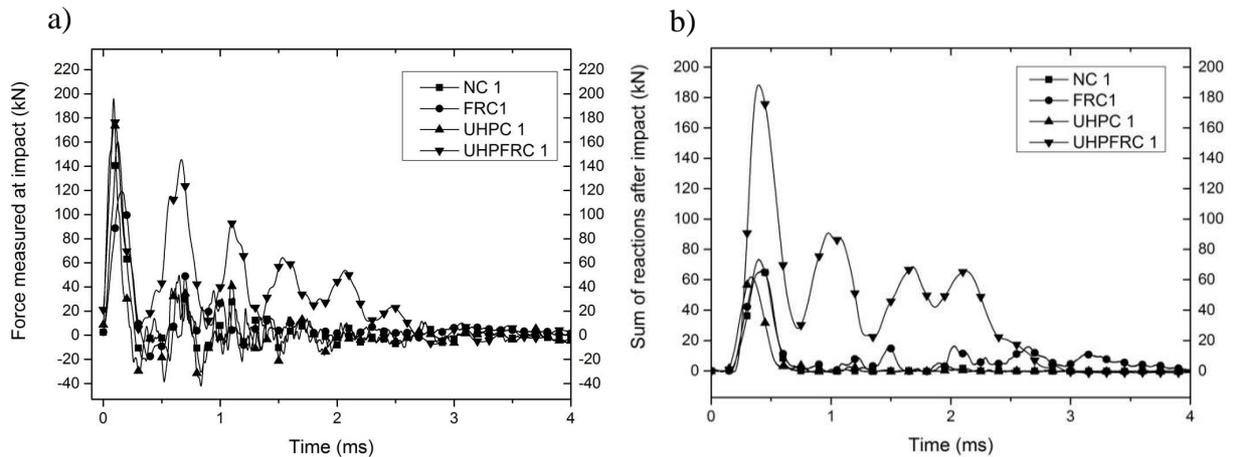
Figure 4. History of forces measured at the a) hammer tip and at the b) supports in first 4 ms after impact.
