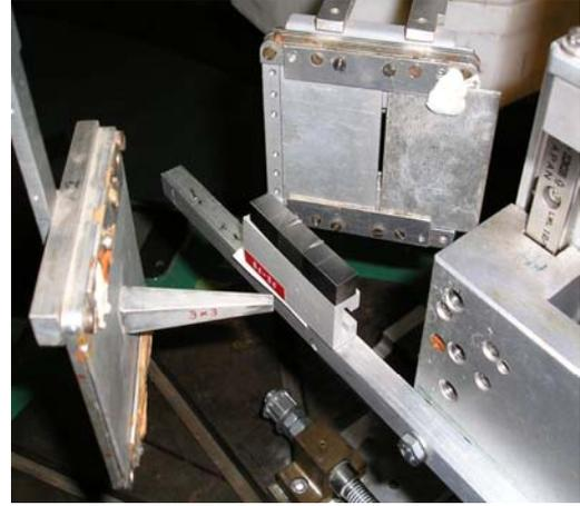
Fig. 2. Photo of the specimen installed on the neutron beam defined by slits.
