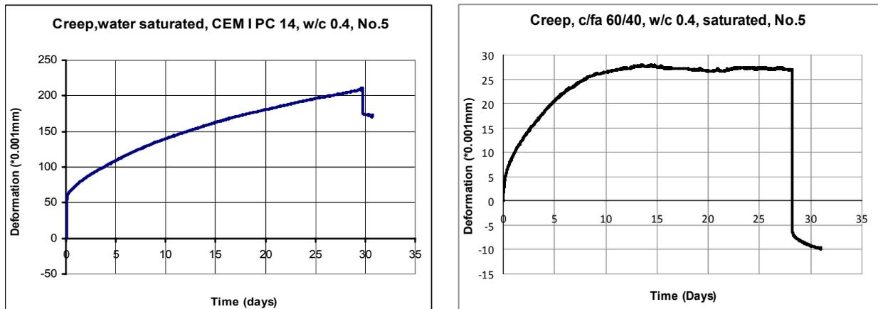
**Fig. 4.** Creep of cement paste with fly ash in 4 months (left) and in 10 months (right) for specimen No.5.
