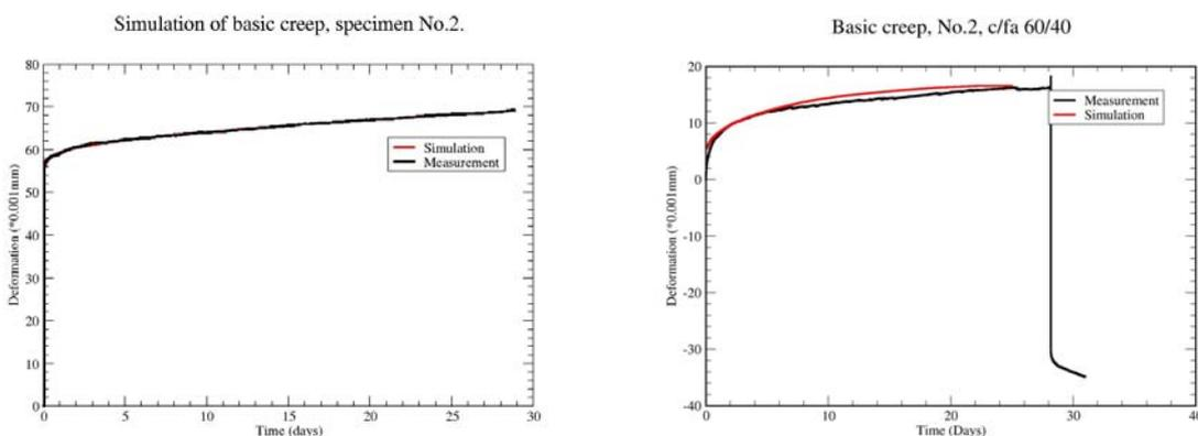
**Fig. 7.** Simulation of basic creep of the specimen No.2. Left picture is for 4 month old material and right picture is for 10 month.
