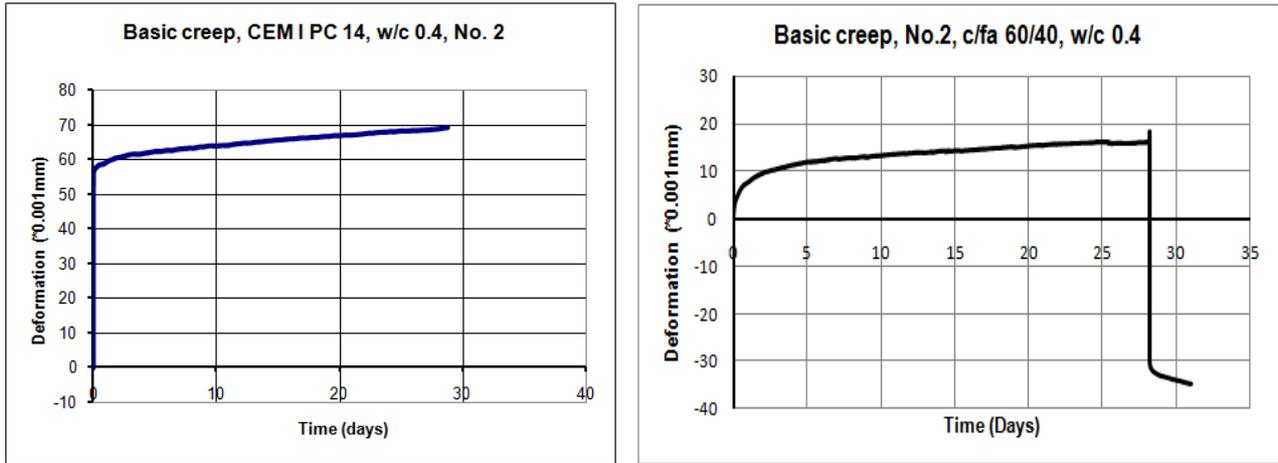
**Fig. 3.** Basic creep of cement paste with fly ash in 4 months (left) and in 10 months (right) for specimen No.2.
