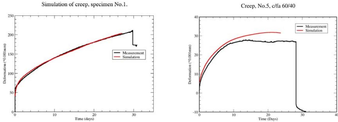
**Fig. 8** Simulation of creep of the specimen No.5. Left picture is for 4 month old material and right picture is for 10 month.
