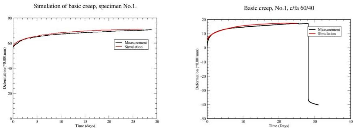
**Fig. 6.** Simulation of basic creep of the specimen No.1. Left picture is for 4 month old material and right picture is for 10 month.
