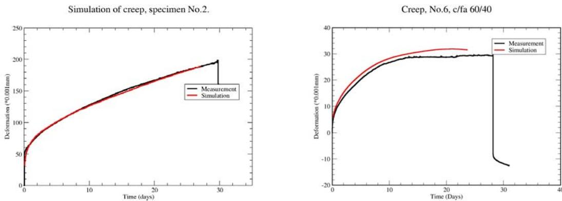
**Fig. 9** Simulation of creep of the specimen No.6. Left picture is for 4 month old material and right picture is for 10 month.
