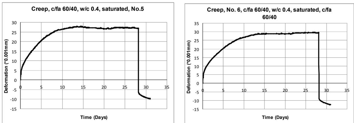
**Fig. 5.** Creep of cement paste with fly ash in 4 months (left) and in 10 months (right) for specimen No.6.
