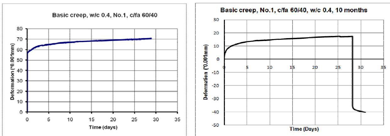
**Fig. 2.** Basic creep of cement paste with fly ash in 4 months (left) and in 10 months (right) for specimen No. 1.
