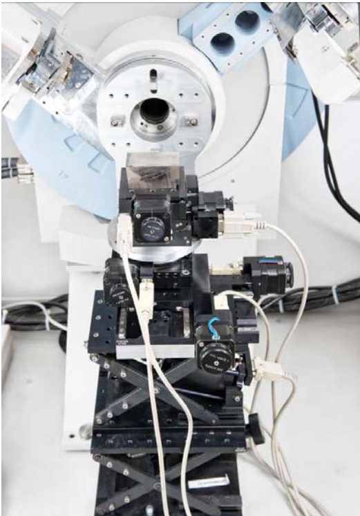
Fig. 1. In-house designed versatile positioning system for XRD analyses of real objects.
