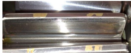
Fig. 16. Contact pattern after 50 000 km.
