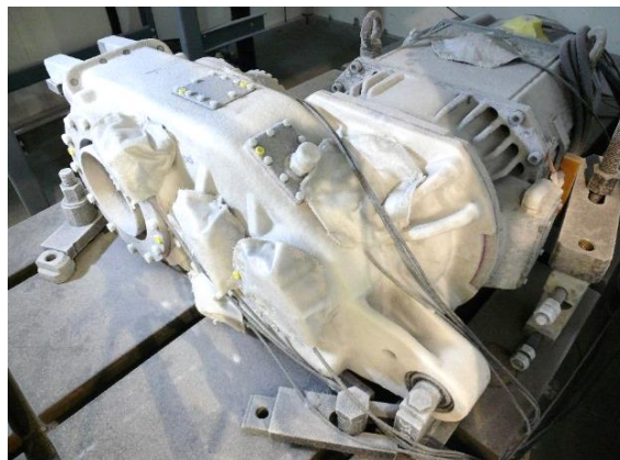
Fig. 10. Cold climate test of assembled gearbox with electro motor and coupling.
