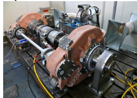
Fig. 6. The really assembled test rig with the location of temperature sensors (EMU gearbox testing in mechanically closed loop).
