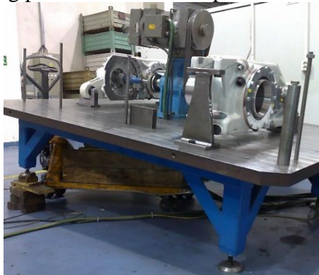
Fig. 3. The test of the tram-gearbox at a cross slope 8^\circ .
