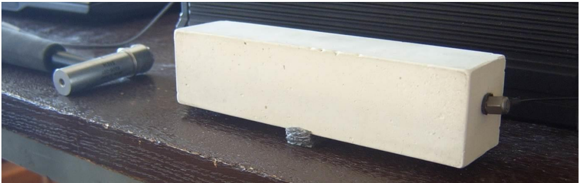
Fig. 1 Test arrangement for the longitudinal vibration
