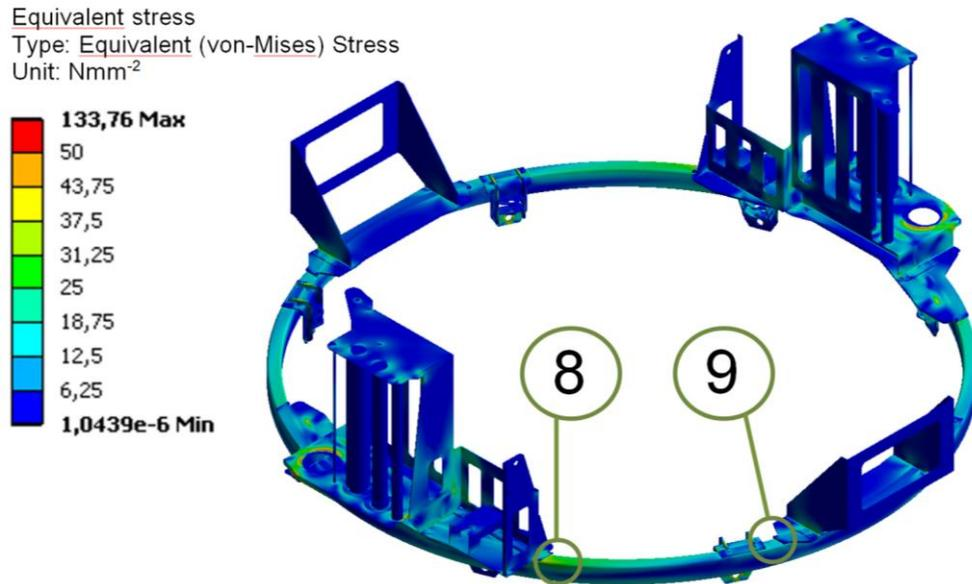
Fig. 3: FEM model of rotating ring.
