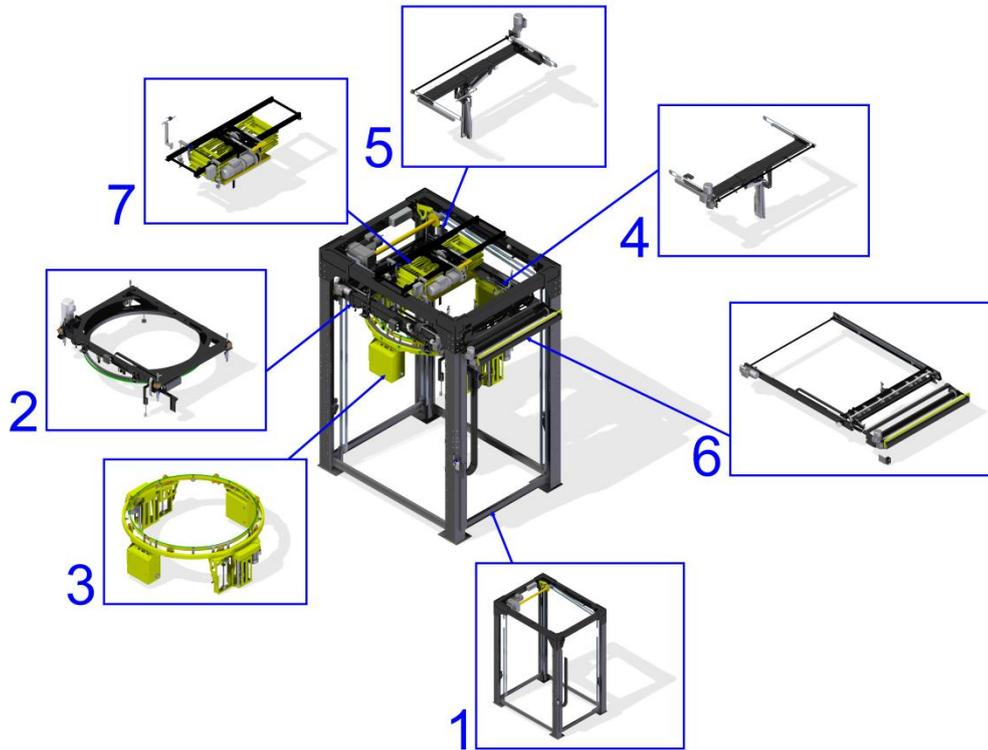
Fig. 1: Division of machine in subassemblies.
