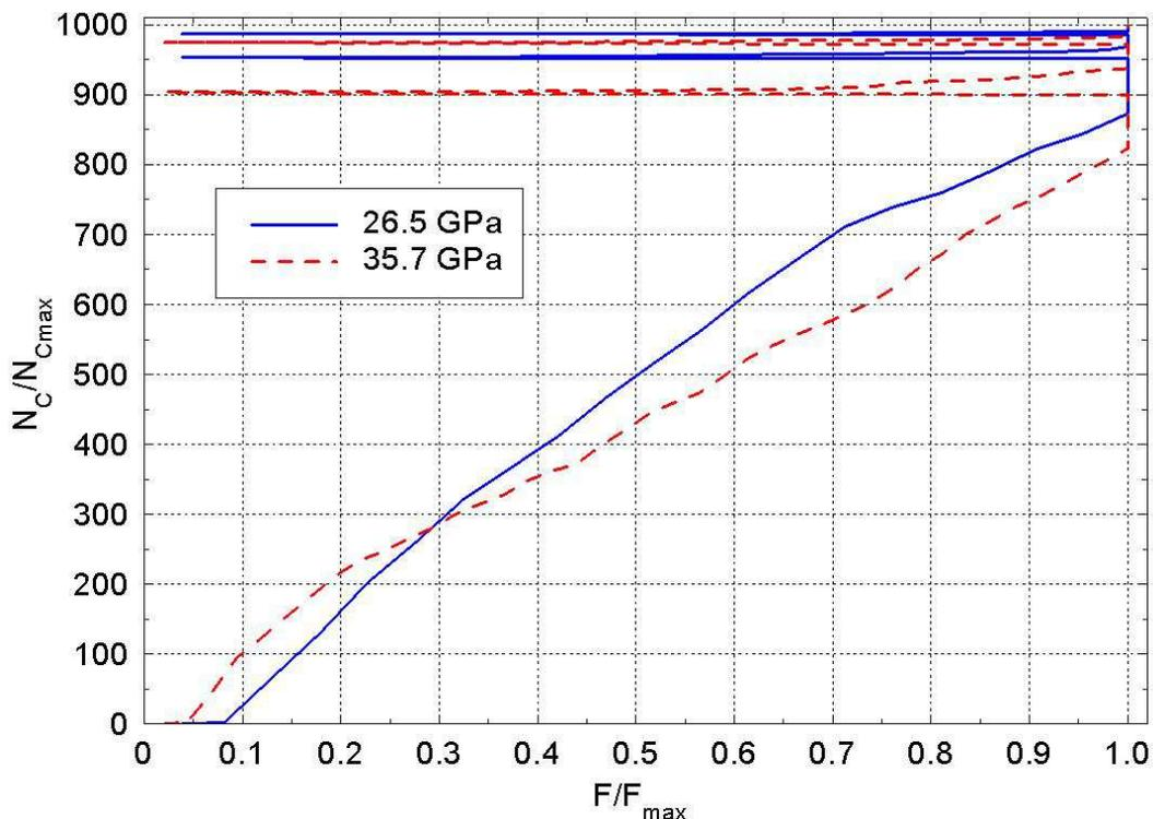
Figure 5: Dependence of the relative cumulative number of overshoots to relative force
