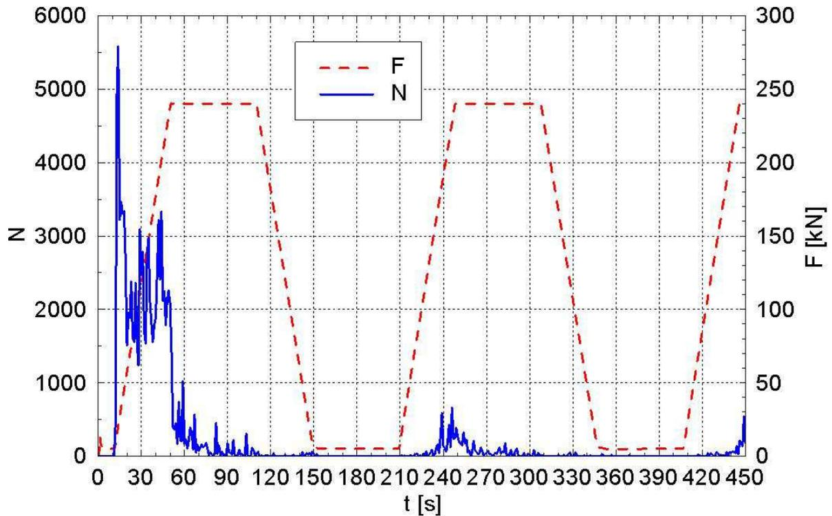
Figure 4: Dependence of the number of overshoots and the forces on time (for sample with  $E_c = 35.7$  GPa)
