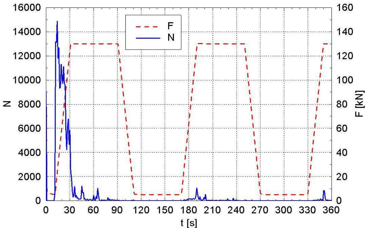
Figure 3: Dependence of the number of overshoots and the forces on time (for sample with  $E_c = 26.5$  GPa)
