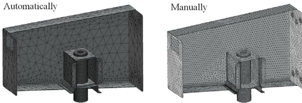
Fig. 4 – Automatically and manually generated mesh
