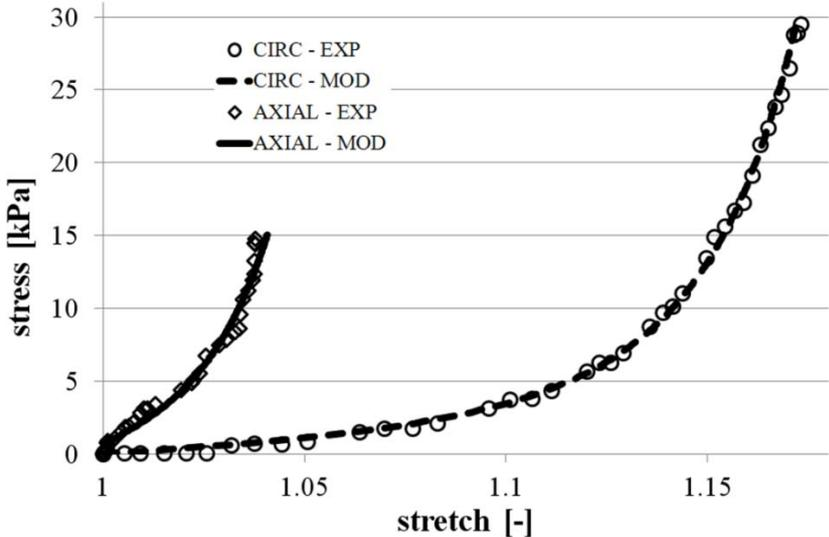
Fig. 3 The experimental data and computed model curves for the sample of the vein. CIRC and AXIAL denote circumferential and longitudinal direction, EXP and MOD denote experimental and model data.
