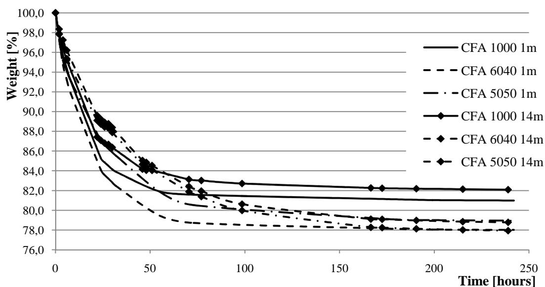
**Fig. 1:** Percentage change in weight of specimens of cement paste with different proportion of fly ash in time due to drying
