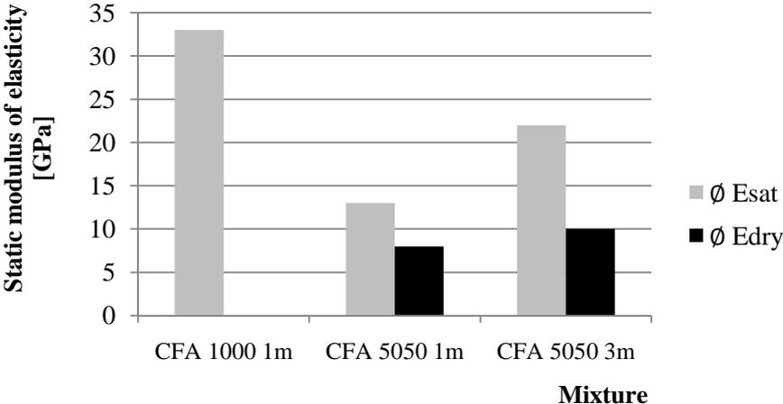
**Fig. 3:** The average values of static modulus of elasticity for each mixture and time
