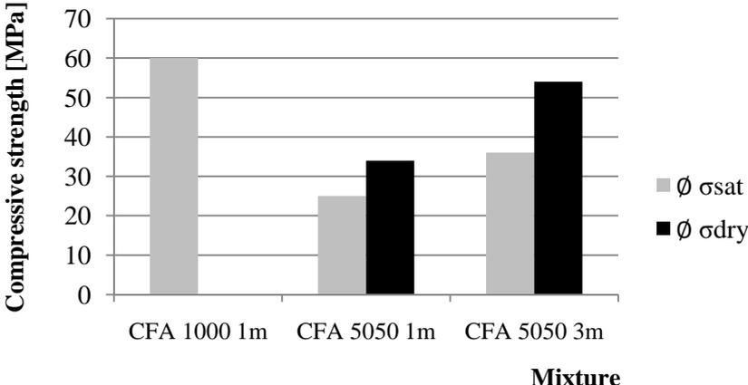
**Fig. 2:** The average values of compressive strength for each mixture and time
