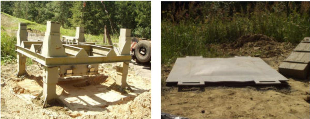
Fig. 1. Experimental equipment – stand and testing plate.
