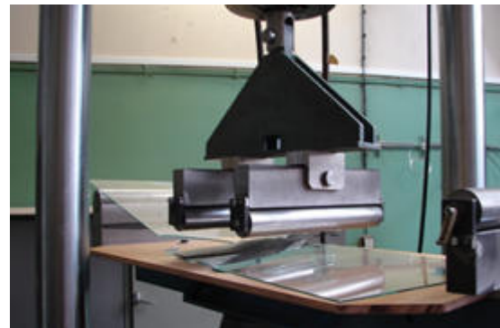
Fig. 2. Broken glass after the test.
