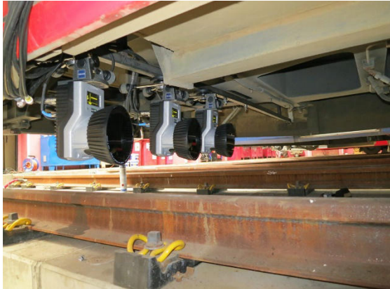
Fig. 4. System of Qualisys cameras mounted to the holder.
