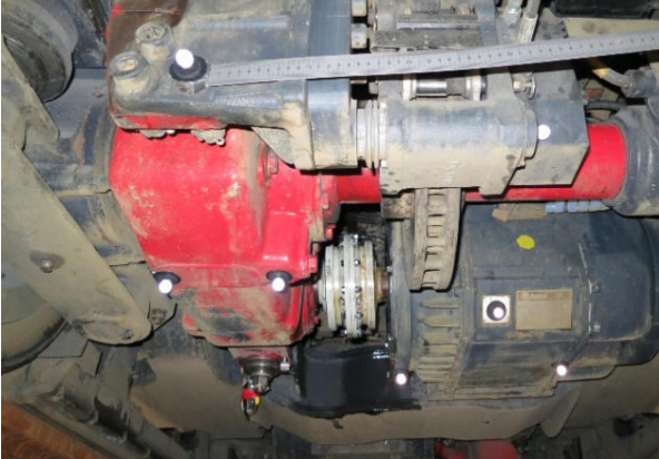
Fig. 3. Markers of the system Qualisys placed on the gearbox and the asynchronous motor.
