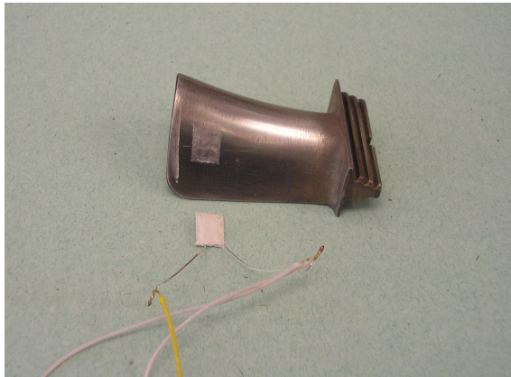
Fig. 1. Failure of the strain gauge mounted with using of the DKS-8 cement.
