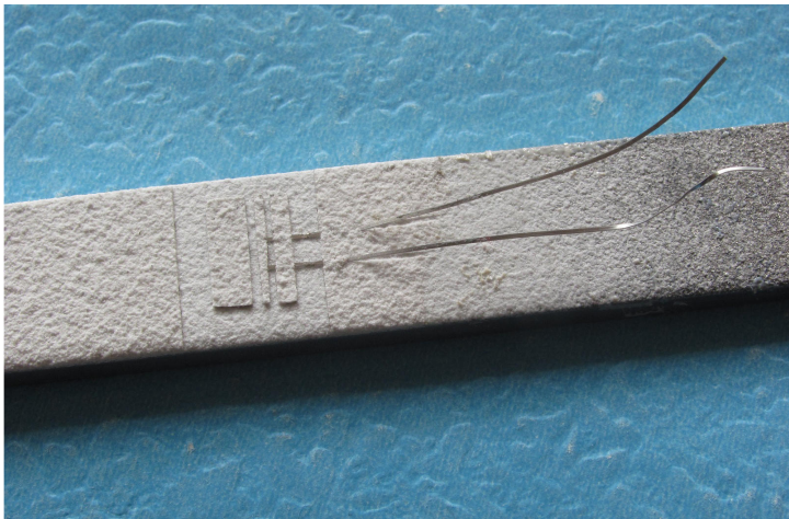
Fig. 7. Strain gauge ZC-NC-1262-120 mounted on the Haynes 230 alloy specimen with using of the ROKIDE technology of flame spraying.
