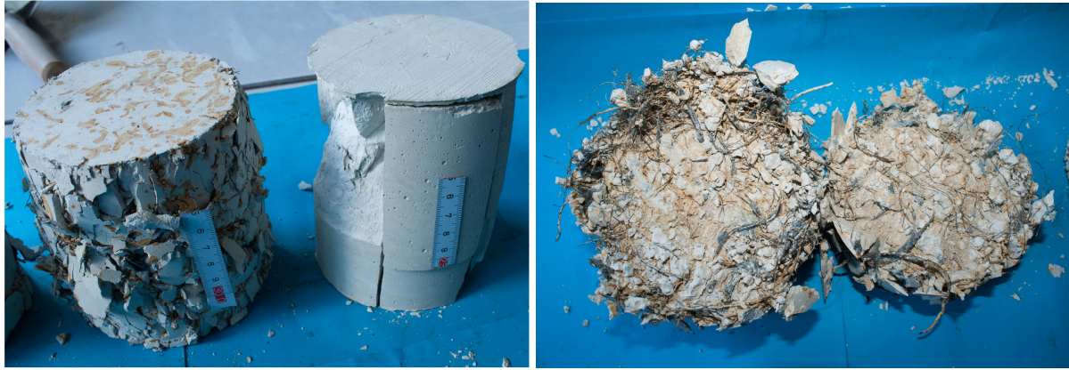
Fig. 1. Compressed samples of the plain G-I (the first from the left) and reinforced samples G-II (the second from the left); typical samples G-II after testing (right).
