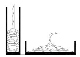
Fig. 3. The influence of the casting of UHPFRC on the fibers distribution.
