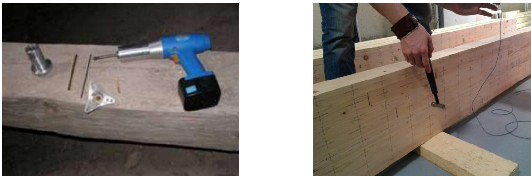
Fig. 4. Examples: a – Specially adapted drill ( http://inspectapedia.com/ ), b – The impact hammer during the measurement.
