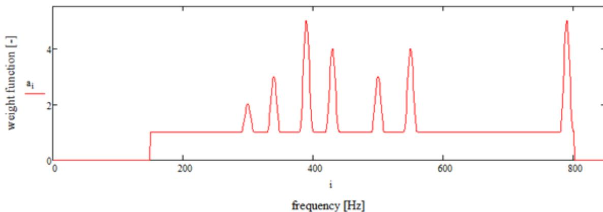
Fig. 2: The weight function for FFT multiplication.
