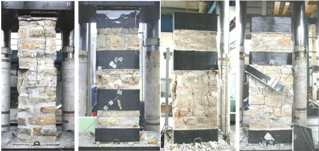
(a) tensile failure of URM column and compressive failure of confined column between CFRP strips
