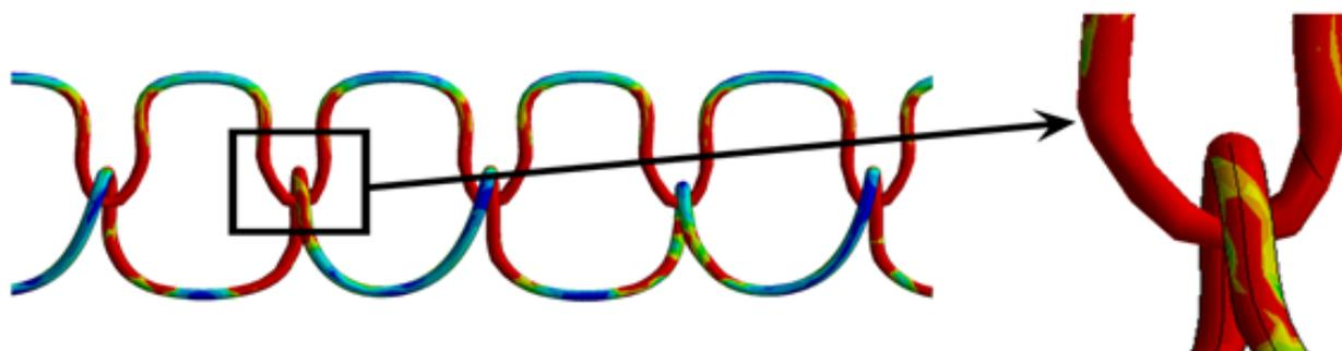
Fig. 11: The observed maximum stress in the contacts of the yarns.
