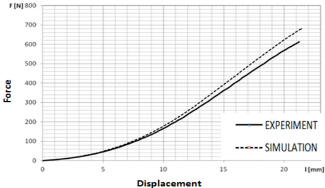
Fig. 15: Graph of dependence of the force  $F$  [N] and deformation  $\Delta l$  [mm].
