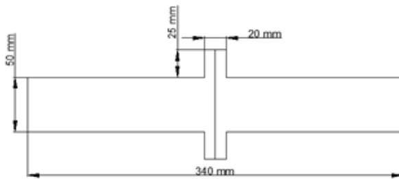
Fig. 1: Shape of the tested specimen.
