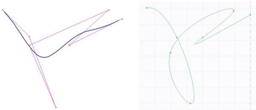
Fig. 8: Comparison of the shape of Bezier (left) and B Spline curve (right) interlaying them through the identical points.
