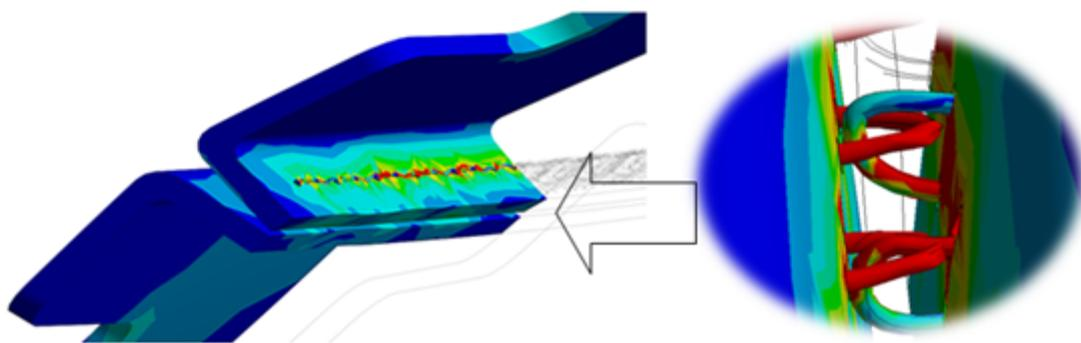
Fig. 14: Sectional view and detail of the observed von-Mises stress in the symmetric half of model.
