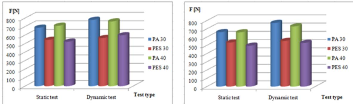
Fig. 5: Changes of seam breaking forces depending on thread and test type (left – in warp direction, right – in the weft direction).
