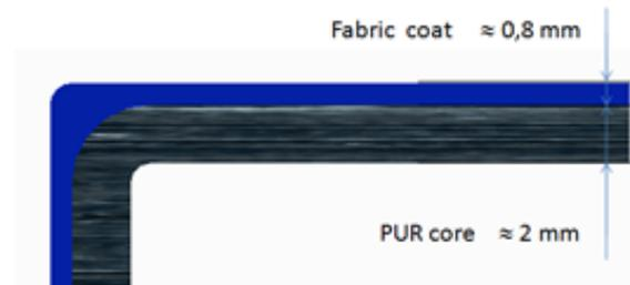
Fig. 2: Layers of the tested sandwich composite.
