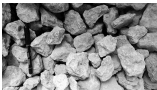
(a) recycled concrete of fraction 32-64 mm
