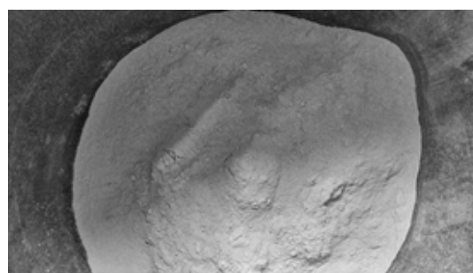
(b) recycled cement powder of fraction 0-0,125 mm
