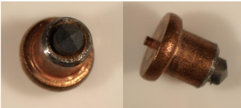
Fig. 1: Sintered tungsten carbide with tetrahedron shape in electrically conductive capsule.
