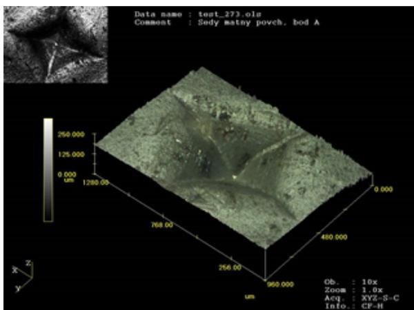
Fig. 4: 3D Detail of imprint of micro tip by microscope.
