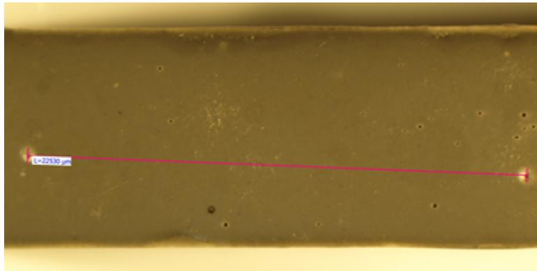
Fig. 6: Microscopy measurement of distance between two imprints.
