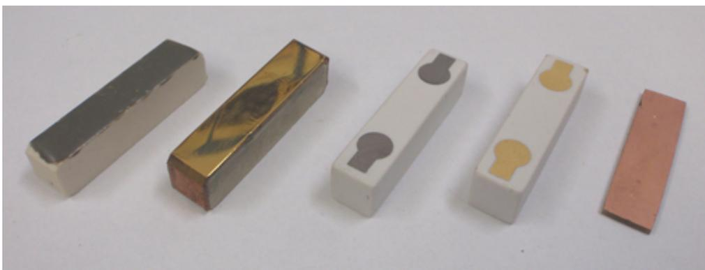
Fig. 2: Impression piece (from left: plastic, gold, titanium, gilded titanium and copper).
