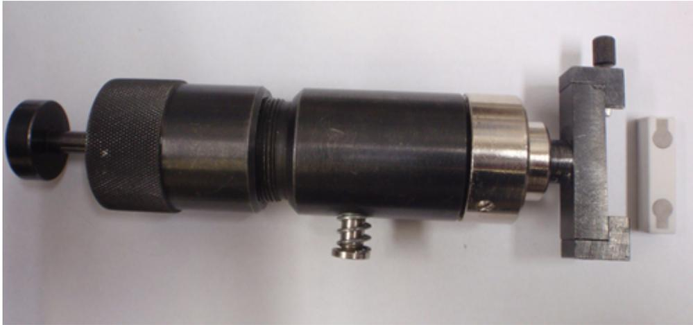
Fig. 3: Spring-operated hammer with impression piece.
