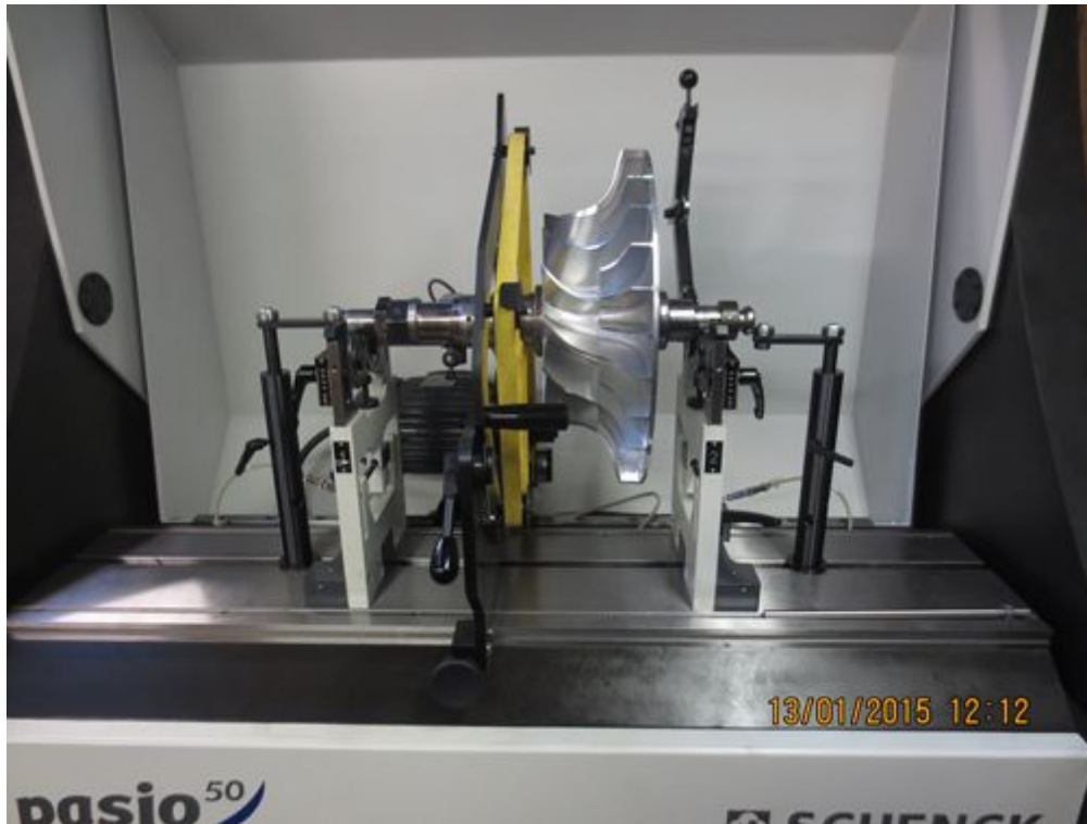
Fig. 1: Low-speed balancing machine.
