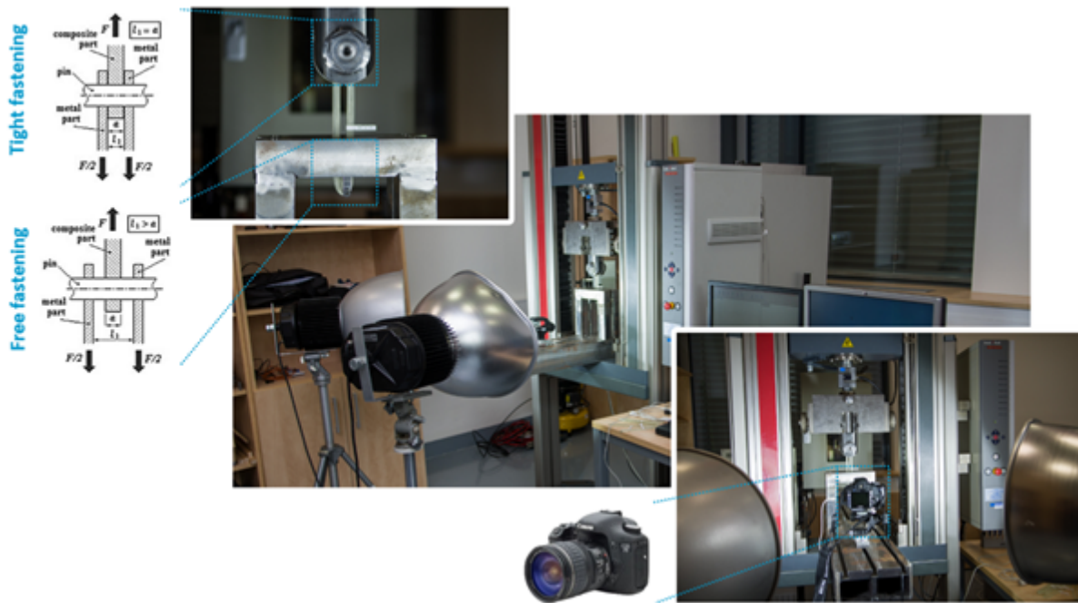
Fig. 4: The process of tensile experimental test of glass fibre wrapping loops – Free fastening.
