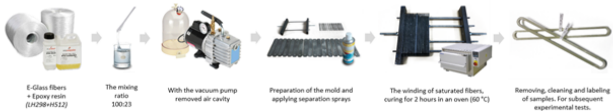
Fig. 2: Manufacturing process of wrapping loops.
