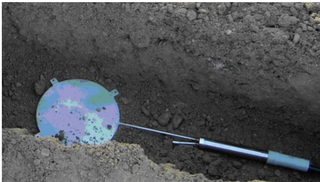
Fig. 2: Pressure sensor of series No. 3500 made by the firm Geokon.
