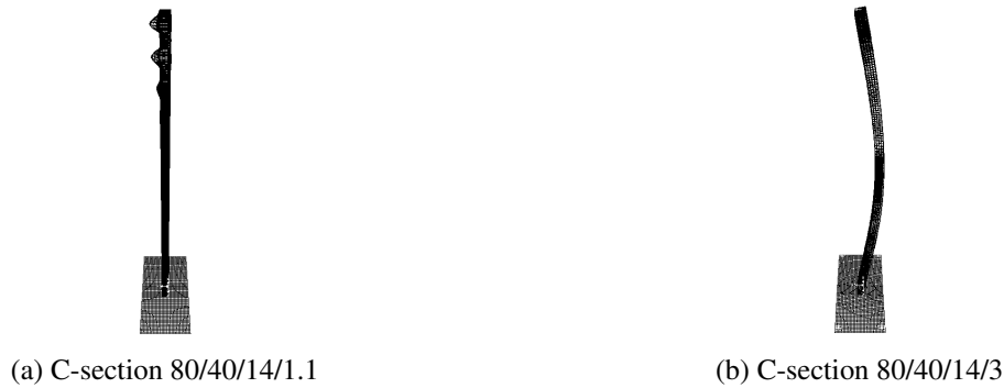
Fig. 6: Deformed shape of thin-walled rod subjected to critical force.
