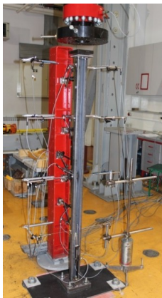
Fig. 3: Thin-walled C section rods prepared for testing.
