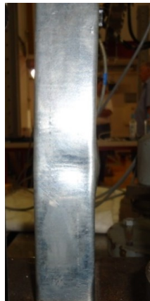
Fig. 4: Local buckling of the web of rod C 80/40/14/1.1.
