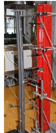
Fig. 5: Loss of stability of rod C 80/40/14/3.
