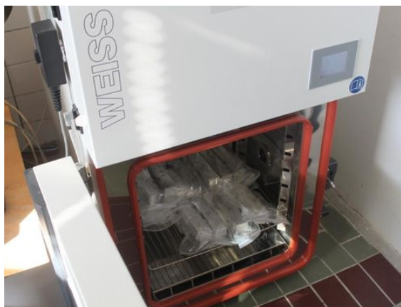
Fig. 1: Climatic chamber of the firm Weiss with specimens of cement-fly ash composites prepared to freeze cycles.
