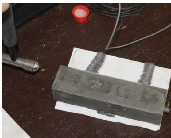
Fig. 2: Measurement system for dynamic modulus determination.
