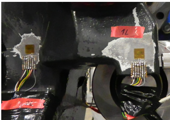
Fig. 2: Strain gauge rosettes installed on the gear box.
