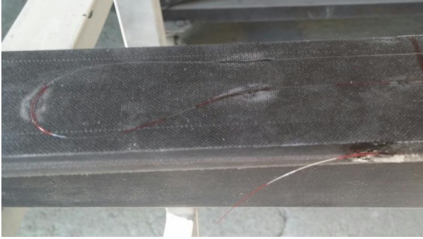
Fig. 4: Detail of optical fiber on the spar cap, just before application of epoxy adhesive.
