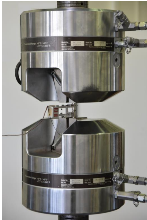
Fig. 6: Experimental setup includes extensometer and hydraulic wedge grips.
