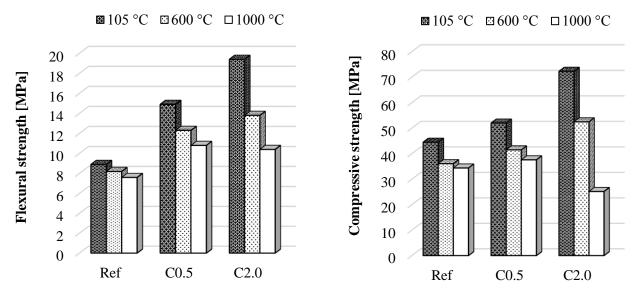
Fig. 1: Values of flexural strength.
