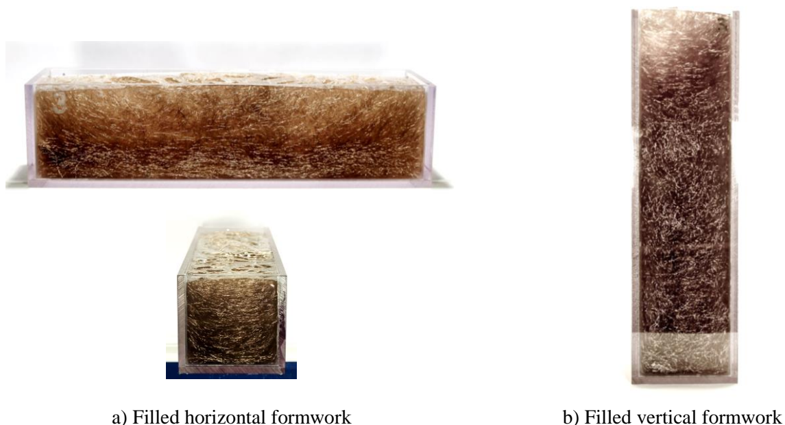
Fig. 3: The orientation of fibers in the matrix of the ultrasound gel after pouring into the transparent formwork.
