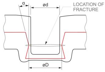
Fig. 4: Simplified scheme of the joint
