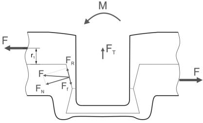
Fig. 4: Computational scheme of the joint
