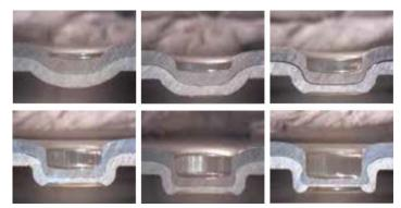
Fig. 1: TOX®-Round Joint formation, [1]
