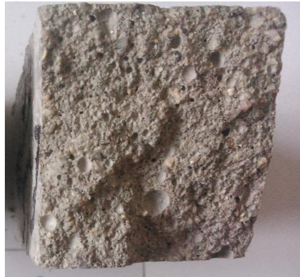
Fine recycled aggregate concrete (FRAC)
