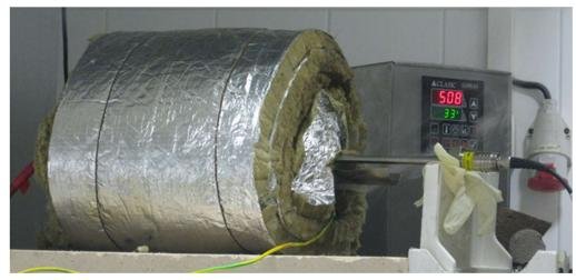
Fig. 1: The temperature loading of the specimen into a special oven and the position of the acoustic emission sensor on the waveguide
