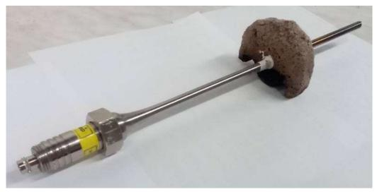
Fig. 2: The acoustic emission sensor on the waveguide
