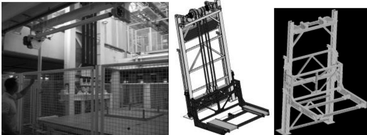
Fig. 1: Real testing of lifting platform (left), CAD model (center) numerical model (right).
