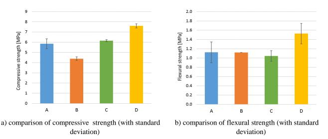
Fig. 2: Comparison of mechanical properties of the 28-day old material/set from destructive tests.
