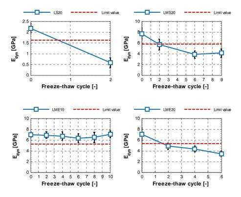
Fig. 1: Evolution of dynamic modulus of elasticity
