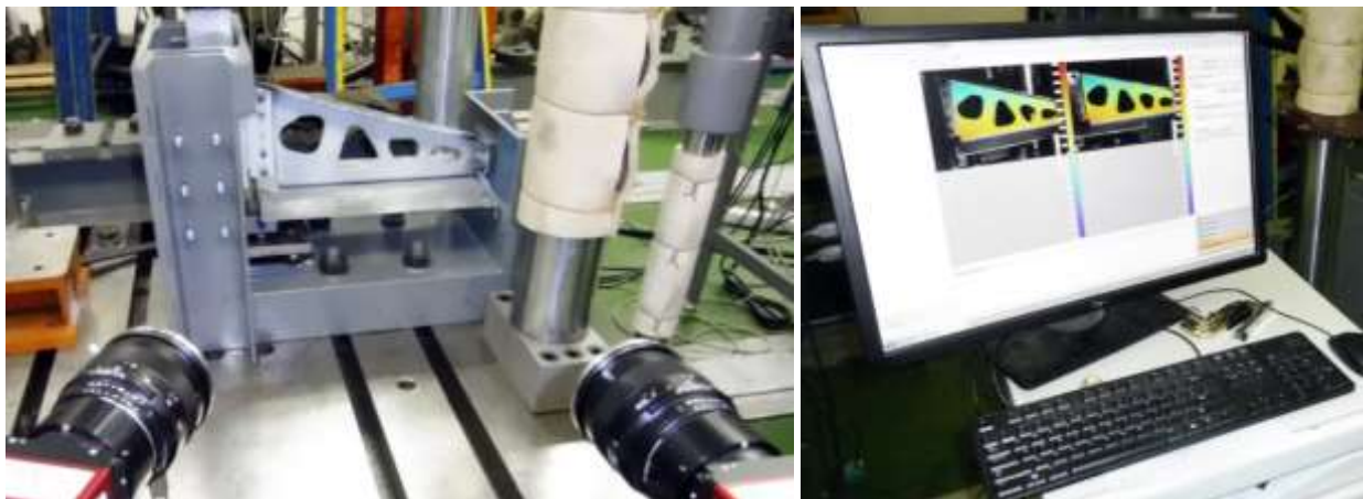
Fig. 3: Test arrangement with cameras of Q-400 image correlation system (left) and results image (right).
