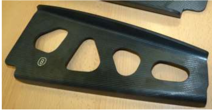
Fig. 1: Thermoplastic composite rib with tailored blanks.
