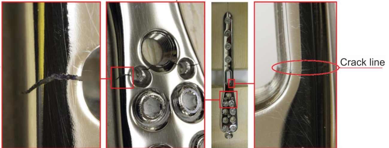
Fig. 6: Results of fatigue test (cracks) for sample no. 1 (locus minoris of the medial plate).
