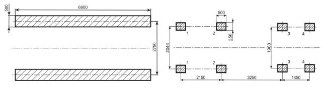
Fig. 2: Geometry and dimensions of contact surfaces of belt carriage with the bridge.
