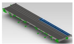
Fig. 5: Boundary conditions for vertical and horizontal loading for position of tank on the boundary of the bridge.
