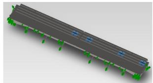
Fig. 7: Boundary conditions for vertical and horizontal loading for position of truck on the boundary of the bridge.
