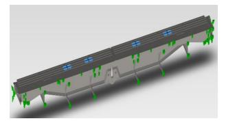
Fig. 6: Boundary conditions for vertical and horizontal loading for position of truck in the middle of the bridge.
