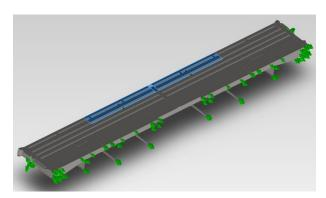
Fig. 4: Boundary conditions for vertical and horizontal loading for position of tank in the middle of the bridge.
