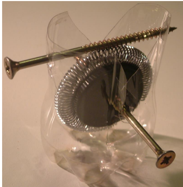
Fig. 6: The experimental model of worm gear - worm thread engages in the coiled tooting of the worm gear.
