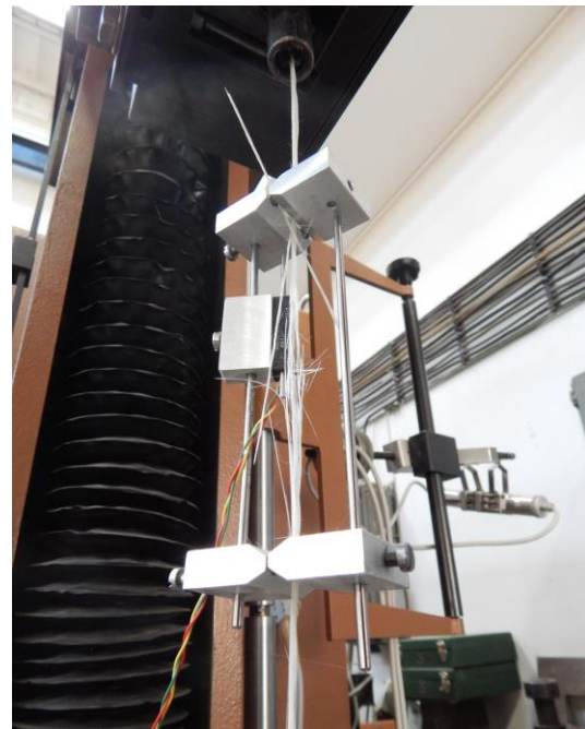
Fig. 2: General view of the specimen in the massive steel sleeves with epoxy inside just after testing.
